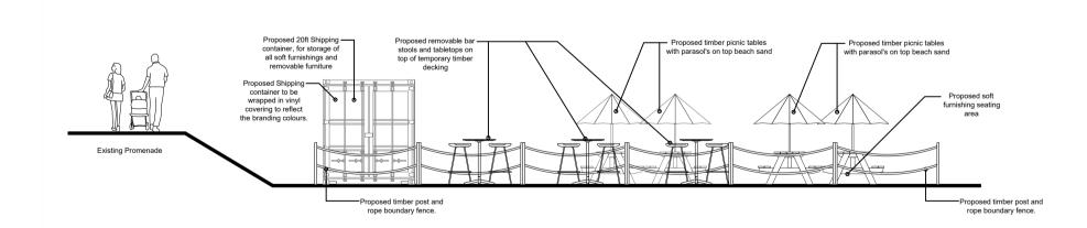
Proposed West Elevation Scale 1:100 @ A1
